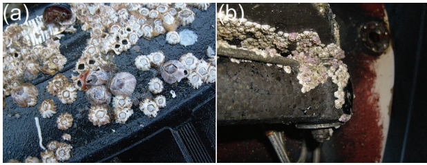
FIGURE 15.7 Biofouling by the barnacles Amphibanalus amphitrite and Elminius modestus in the port area of Saint Malo (North Brittany). (a) Tire used as port fender, (b) Underside of a boat needing cleaning.
