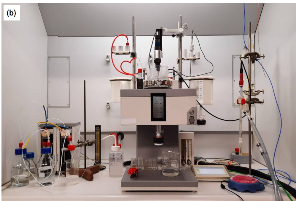
Figure S1. Schematic representation of the automated reactor used for the synthesis of the materials of this study and adapted with a Raman probe for in situ monitoring experiments (a) and photograph of the experimental setup (b).
