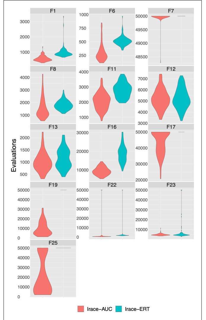
Fig. 5. Violin plots of first hitting times for the configurations found by Irace when tuning for ERT and AUC, respectively, for problems on which Irace-AUC outperforms Irace-ERT . Results are from the 100 independent validation runs. Targets are listed in Tab. I, and the configurations of the GAs can be found in Tab. II. For each run, values are capped at the budget 50 000 if the algorithm cannot find the target.
