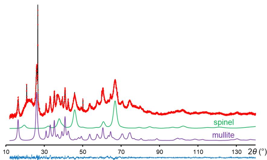
Fig. 1. Rietveld plot for sample SP\_1080\_1h:  $i_{obs}$  (red dots),  $i_{calc}$  (black),  $i_{obs} - i_{calc}$  (blue), and contributions of the spinel phase (green) and mullite (purple). Sharp peaks correspond to quartz. Sample holder baseline subtracted.
