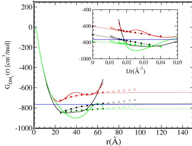
Fig.1B. Finite size scaling analysis of KBI for  $x=0.7$ , for the 3 independent runs shown in Fig.9 with the same 3 color conventions. The inset shows the  $1/r$  dependence which obeys Eq.(2B). Corresponding RKBI are shown both in the main panel and inset. Close dots correspond to points  $r < L/2$ , and open dots for  $r > L/2$ . The horizontal blue line is the experimental value.
