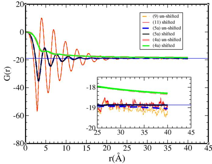
Fig.1C. Comparison of the calculation methods for the RKBI for a Lennard-Jones liquid (see text). The lower inset is a zoom on the tail behaviour of the various  $G(r)$  of the main panel. In both plots, the thin horizontal blue lines serves as a guide for the correct KBI value.
