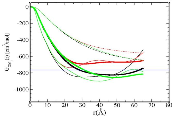
Fig.2C. Comparison of the calculation methods for the RKBI for  $x=0.7$  for 3 different runs depicted with 3 colors (black, red, green). The data from Eq. (2C) are shown as thin dashed lines, that for Eq.(3C) in thick lines, and that from Fig.9 in thin lines. The horizontal blue line is the data the experimental KBI value.
