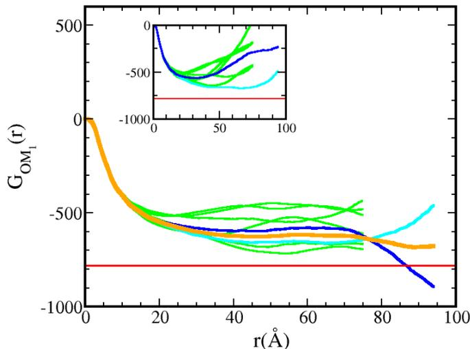
Fig.1A. Comparison of the RKBI for a  $N=32000$  system (blue and cyan curves) with that of the  $N=16000$  systems shown in Fig.11 (reproduced in green here). The inset shows the original asymptote uncorrected curves. The average of the 2 runs for the larger system is shown as orange curve.
