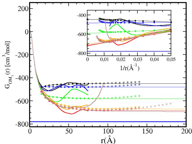
Fig.2B. Finite size scaling analysis of KBI for  $x=0.2$ , for the independent runs shown in Fig.11 with the same color conventions. In addition, one result for the  $N=32000$  particle of Fig.1A is equally shown as brown lines and symbols. Line and symbol conventions are as in Fig.1B.
