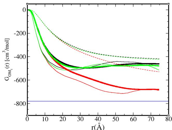
Fig.4C. Comparison of the calculation methods for the RKBI for  $x=0.2$  for 3 different runs, and computed from the shifted correlation functions. The horizontal blue line is the data the experimental KBI value.
