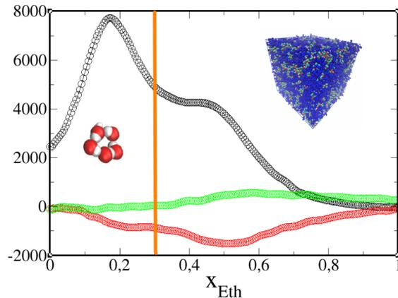
Figure 8: Illustration of the two ethanol concentration regions for each extremum of the KBI, separated by  $x = 0.3$  (vertical orange line). Left part for  $x < 0.3$  concerns ethanol micellar entities, while right part  $x > 0.3$  concerns standard micro-segregated ethanol-heptane domains.
