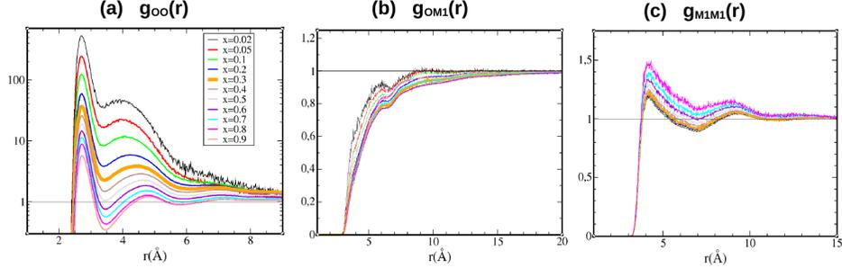
Figure 7: Ethanol concentration dependance of selected atom-atom pair correlation functions. **(a)** Ethanol oxygen-oxygen pair correlation functions  $g_{OO}(r)$ ; **(b)** ethanol oxygen heptane 1st carbon group cross correlations  $g_{OM_1}(r)$ ; **(c)** heptane 1st carbon group correlations  $g_{M_1M_1}(r)$ . The ethanol concentration  $x = 0.3$  is marked at thicker orange line.
