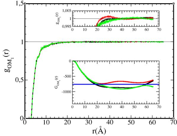
Figure 9: Long range tail contribution for ethanol-heptane cross correlation function  $g_{OM_1}(r)$  for ethanol concentration  $x = 0.7$  shown in the main panel for 3 different runs of 5ns each. The upper inset is a close-up of the tail part. The lower inset shows the respective RKBI  $G_{OM_1}(r)$  functions, along with the experimental KBI (in blue).
