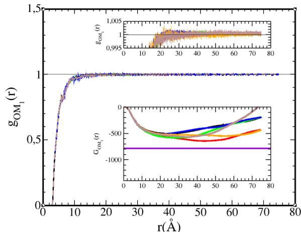
Figure 10: Long range tail contribution for ethanol-heptane cross correlation function  $g_{OM_1}(r)$  for ethanol concentration  $x = 0.2$  shown in the main panel for 5 different runs of 5ns each. The upper inset is a close-up of the tail part. The lower inset shows the respective RKBI  $G_{OM_1}(r)$  functions, along with the experimental KBI (in purple).
