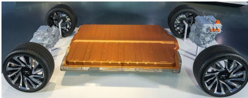
General Motors concept reveal in 2020: 200 kWh Li-Battery (800 volts, 350 kW charging)
