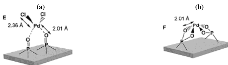
Figure 4. Proposed surface structures around Pd(II) center of (a) PdHA-0 and (b) PdHA-1. Source: [38]. Adapted with permission of American Chemical Society.
