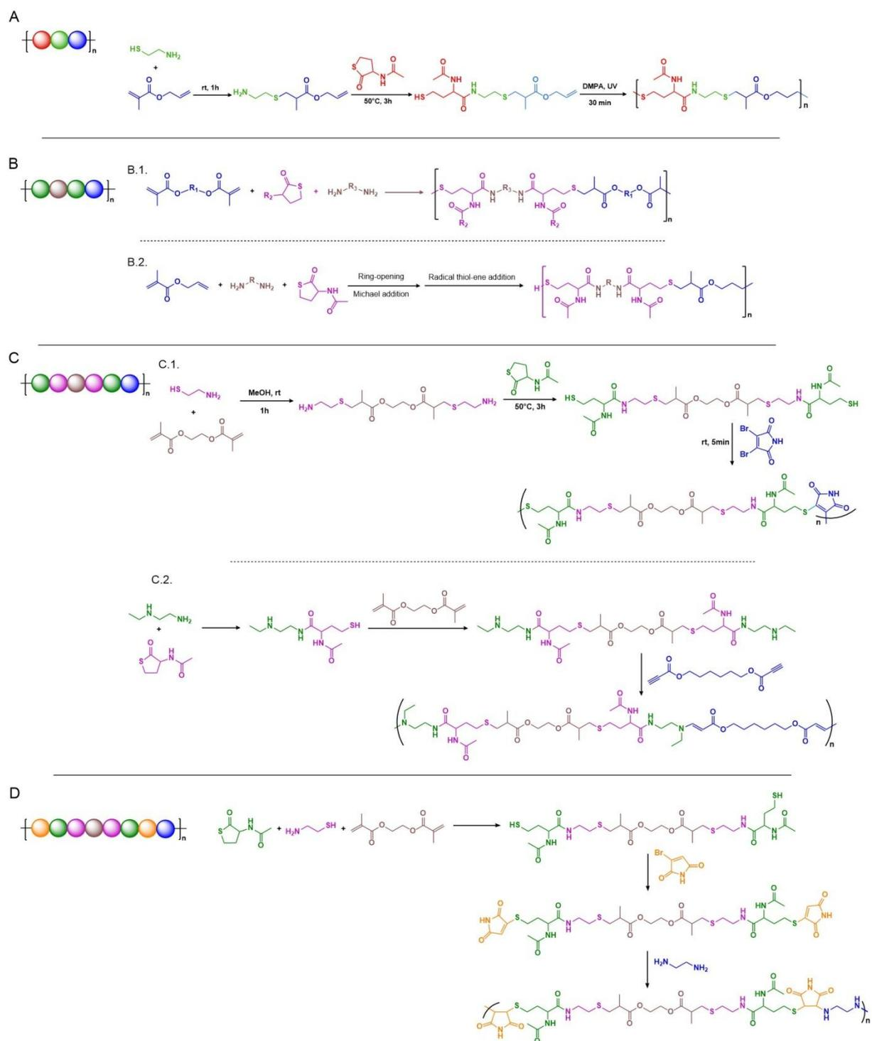
**Figure 19.** Different strategies using thiolactone chemistry for the synthesis of periodic macromolecules.<sup>144-148</sup>
