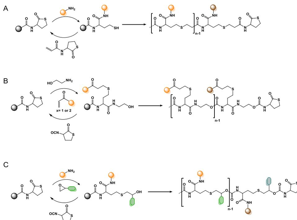
**Figure 21.** Different strategies based on thiolactone chemistry for the synthesis of sequence-defined macromolecules.<sup>151, 152, 158</sup>
