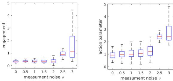
Fig. 6. Performance for increasing noise  $\sigma$ . Left: Engagement mean absolute deviation from its maximum value (10). Right: Action parameter mean absolute deviation from its optimal value (5). The measurement noise has  $\sigma = 1$ .
