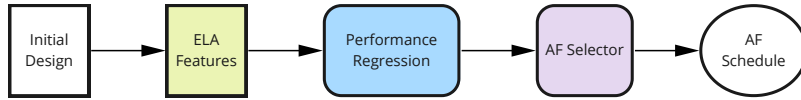
Figure 1: How to select acquisition function (AF) schedules Based on the evaluated initial design of a BO run, we compute the ELA features. With those we query a trained RF and observe the predicted performance of each AF schedule. The Acquisition Function Selector returns the AF schedule with the best predicted performance to use for surrogate-based evaluations.
