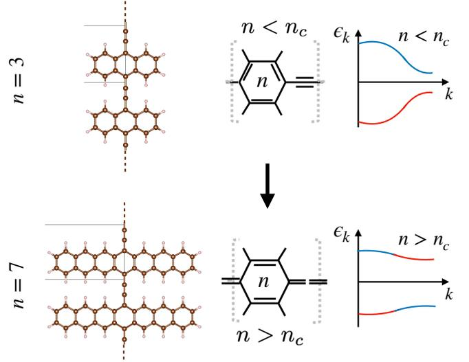
FIG. 1. Topological phase transition of polyacene polymers: as the acene length  $n$  increases, the bridge configuration switches from ethylnic ( $-C \equiv C-$ ) to cumulenic ( $=C=C=$ ), while the central ring goes from an aromatic to a quinoidal form. Above a critical length  $n_c$ , the topologically non-trivial phase (see text) emerges, showing a smooth change of orbital character (red, blue) across the Brillouin zone (band inversion).
