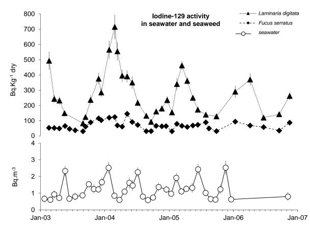
Figure 7: lodine-129 activity in seawater and in brown seaweed collected in Goury, near the outlet of the ORANO reprocessing plant in La Hague. Error bars account for metrological uncertainties (2 x sigma; may be masked by symbol).
