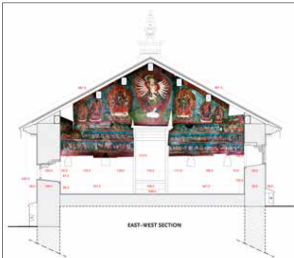
Fig. 4. East-West section of Śāntipur Temple vestibule's South wall before the earthquakes of 2015 © Pierre Gérard Bendele, Ludovic Dusuzeau/UNESCO Kathmandu, paintings images: courtesy of A. von Rospatt
