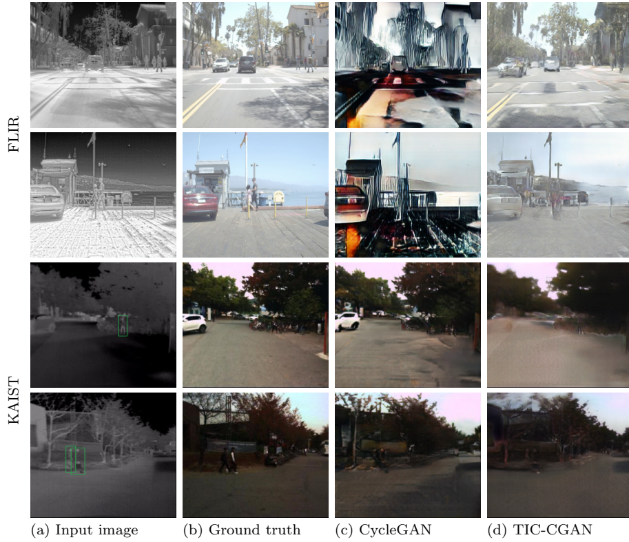
Fig. 3 Qualitative results of CycleGAN [48] and TIC-CGAN [2] on two sample thermal images (the input) with their corresponding visible images (the target) for each dataset. From top to bottom: results of 4 sample images, two first rows showing results on FLIR dataset and the two last rows on KAIST dataset. For each sample image, annotations of target objects present in the input thermal images are drawn with green bounding boxes.
