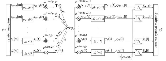
Fig. 1. FDA-based spatial data focusing baseband system model
