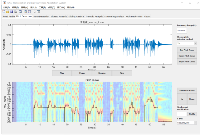
(a) Pitch detection for debleeded first string vibration signal of Jasmine Flower recordings
