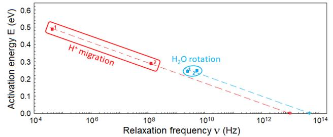
**Figure 7.** Activation energies  $E_a$  (eV) vs. relaxation frequencies  $\nu$  (Hz) at 293 K attributed to proton migration (hopping) and water rotation in *pristine* (1) and *Zn-titanate* (2):  $E = 2.3kT \log \nu_0 - 2.3kT \log \nu$ . The slope of dotted lines is  $2.3kT$  and gives the average frequency prefactors (attempt frequencies)  $\nu_0$  of about  $10^{13}$  and  $5 \cdot 10^{13}$  Hz for proton migration (red) and water rotation (blue), respectively.
