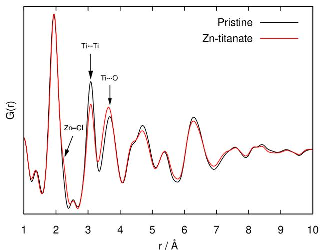
**Figure 3.** X-ray PDFs of *pristine* and *Zn-titanate*.
