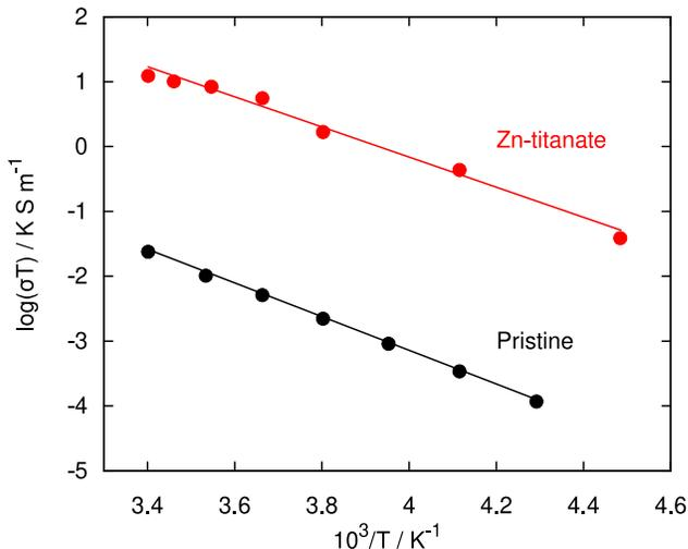
**Figure 2.** Arrhenius plot of the bulk conductivities for the *pristine* and *Zn-titanate*.
