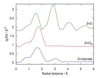
**Figure 4.** Fourier transform Zn K-edge EXAFS oscillations of *Zn-titanate* and for comparison ZnO and ZnCl<sub>2</sub>.
