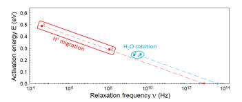
**Figure 7.** Activation energies Ea (eV) *vs.* relaxation frequencies v (Hz) at 293 K attributed to proton migration (hopping) and water rotation in *pristine* (1) and *Zn-titanate* (2):  $E = 2.3kT \log v_0 - 2.3kT \log v$ . The slope of dotted lines is 2.3kT and gives the average frequency prefactors (attempt frequencies)  $v_0$  of about  $10^{13}$  and  $5\times10^{13}$  Hz for proton migration (**red**) and water rotation (**blue**), respectively.
