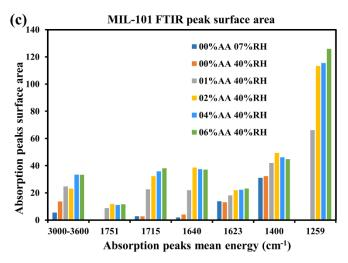
**Figure 4** FT-IR spectra of thin films of a) MIL-101(Cr),b) UiO-66(Zr)-2CF<sub>3</sub> exposed to water/AA vapors of different composition acquired by using IR ellipsometer and c) FT-IR absorption bands surface area obtained from IRVASE spectra. Extinction coefficient are determined with a precision of 0.001
