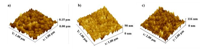
Figure 1. AFM images of a) MIL-101(Cr), b) UiO-66(Zr)-2CF<sub>3</sub>, c) ZIF-8(Zn) thin films
