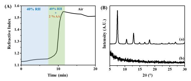
**Figure 2.** (A) RI evolution of ZIF-8(Zn) thin films exposed to sequential different environments namely 40% RH, 2% of AA and 40% RH and dry air. (B) PXRD pattern of ZIF-8(Zn) films (a) before and (b) after exposure to AA/water vapors.
