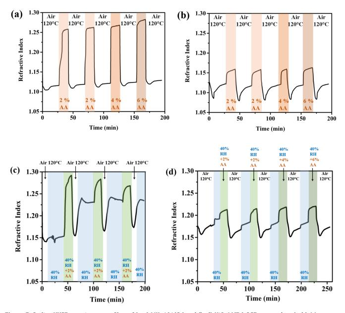
**Figure 5.** Cycling UVSE experiments on films of (a, c) MIL-101(Cr) and (b, d) UiO-66(Zr)-2CF<sub>3</sub> exposed to (a, b) AA vapors (2, 4 or 6 %  $P/P_{vapsat}$ ) or desorption steps (120°C, 2 min, 18°C/min) or (c, d) water vapor at 40%RH, water (RH 40% RH) and AA (2, 4 or 6 %  $P/P_{vapsat}$ ) vapors and desorption steps (120°C, 2 min, 18°C/min).
