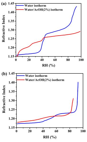
**Figure 3.** Water adsorption isotherm of (a) MIL-101(Cr) film and (b) UiO-66(Zr)-2CF<sub>3</sub> films exposed to water vapors (RH 40%) and a mixture of water vapors at 40% RH and AA vapors at 2%  $P/P_{vapsat}$ . Refractive index is given at 700 nm wavelength.
