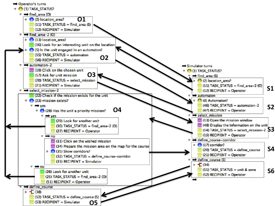
Fig. 6. Partial model of the operator and simulator interaction
