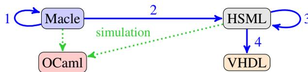
Fig. 6 Compilation flow of Macle to VHDL
