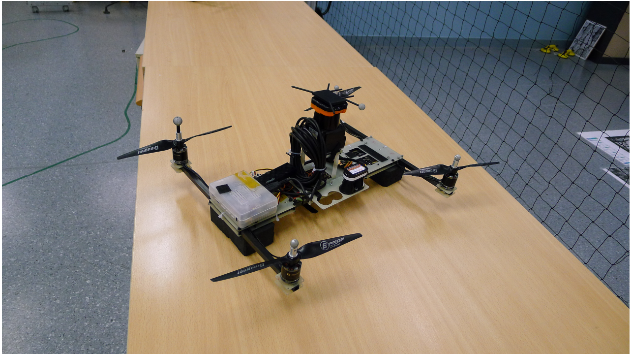
Figure 2: Quadrotor developed at ISIR, equipped with a Hokuyo URG-30LX 2D LiDAR, an MPU6000 3 axis accelerometer/gyrometer unit and an SF10/A laser altimeter from Lightware Optoelectronics.
