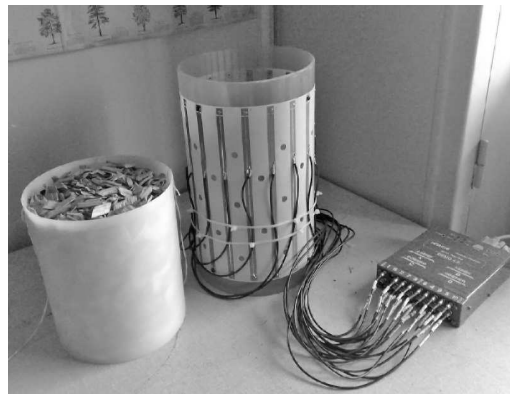
Figure 2: ECT sensor formed by a set of wire electrodes and dedicated to the measurement of water content in wood-chips.
