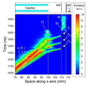
Figure 7. Space—time emission diagram obtained from fast ICCD imaging to highlight the self-organized guided streamers ( $\alpha$ ,  $\theta$ ,  $\gamma$ ) and decipher their mechanisms of propagation and interaction with MM and MP targets.  $\Pi$ : residual surface discharge,  $\Delta$ : dark domains where leaders are assumed to be formed,  $\Theta$ : primary ionizing event in the inter-target region,  $\Phi$ : filamentary discharge.
