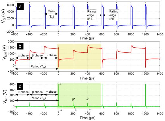
Figure 11. Time profiles of (a) the voltage delivered by the generator with the following set parameters: A = 5 kV,  $f_{rep} = 5 \text{ kHz}$ ,  $D_{\text{Cycle}} = 10 \%$ , (b) the voltage measured on the metal mesh target, (c) the voltage measured on metal plate target.
