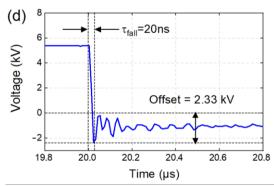
Figure 2. (a) Ideal positive square pulse, (b) real positive square pulse obtained with the HV power supply, (c) enlarged view of the pulse rising edge to evidence  $\tau_{rise}$ , overshoot and ringing, (d) enlarged view of the pulse falling edge to evidence  $\tau_{fall}$  and backswing.
