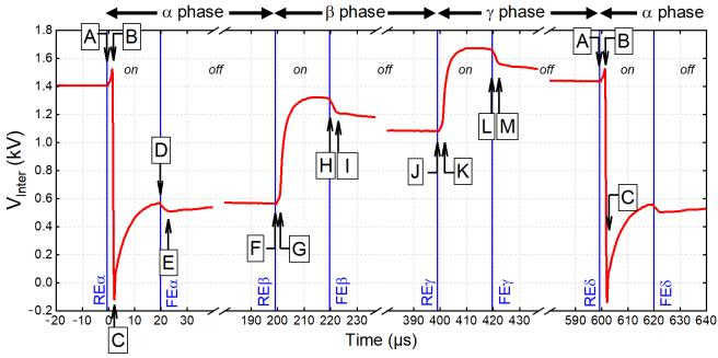
Figure 15. Time profile of the voltage measured in the inter-target region. The three phases correspond to the self-organization of three guided streamers (A = 5 kV,  $f_{rep} = 5 \text{ kHz}$ ,  $D_{Cycle} = 10 \%$ ). RE and FE stand for rising edge and falling edge, respectively.
