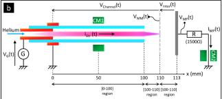
Figure 1. (a) CHEREL-MM-MP configuration. The CHEREL (Capillary with inner Hollow Electrode and outer Ring Electrode) generates a jet of cold plasma that interacts with MM (metal mesh target) and MP (metal plate target) placed in series, (b) Equivalent electrical schematics of (a) including voltage generator, electrical probes and resistor for electrical characterizations.
