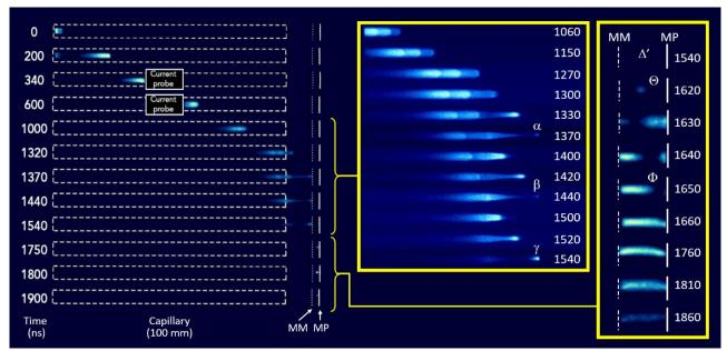
Figure 6. Fast ICCD pictures of positive guided streamers ( $\Omega$  = 3) propagating in the CHEREL's capillary, then interacting with ambient air, metal mesh (MM) target at floating potential and metal plate (MP) target connected to R=1.5 k $\Omega$  that is grounded (A = 5 kV,  $f_{rep}$  = 5 kHz,  $D_{Cycle}$  = 10%).
