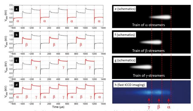
Figure 8. Time profiles of the voltage measured in the MM target considering (a)  $\alpha$ -phase highlighted, (b)  $\theta$ -phase highlighted, (c)  $\gamma$ -phase highlighted, (d) all phases highlighted. Schematic view of a train of (e)  $\alpha$ -streamers, (f)  $\theta$ -streamers, (g)  $\gamma$ -streamers. (h) Fast ICCD imaging picture of three self-organized guided streamers trains.
