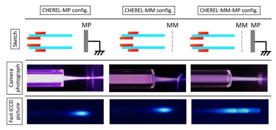
Figure 3. Pictures obtained by digital photography and by fast ICCD imaging, considering the CHEREL-MP configuration (train of repeated guided streamers), the CHEREL-MM configuration (train of repeated guided streamers) and the CHEREL-MM-MP configuration (train of self-organized guided streamers).
