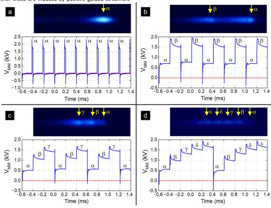
Figure 5. Spatial profiles of self-organized guided streamers measured by fast ICCD imaging and time profiles of the voltage measured on the MM target for (a)  $\Omega$  = 1, i.e., no self-organization, (b)  $\Omega$  = 2, (c)  $\Omega$  = 3 and (d)  $\Omega$  = 5. The symbols  $\alpha$ ,  $\beta$ ,  $\gamma$ ,  $\delta$  and  $\varepsilon$  represent the self-organizing states in order of appearance.
