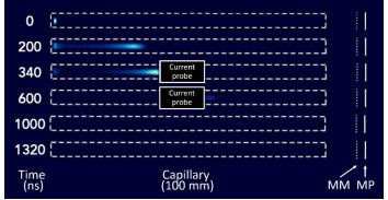
Figure 10. Fast ICCD pictures of negative guided streamers propagating in the CHEREL's capillary (A = 5 kV,  $f_{rep} = 5 \text{ kHz}$ ,  $D_{\text{Cycle}} = 10\%$ ).
