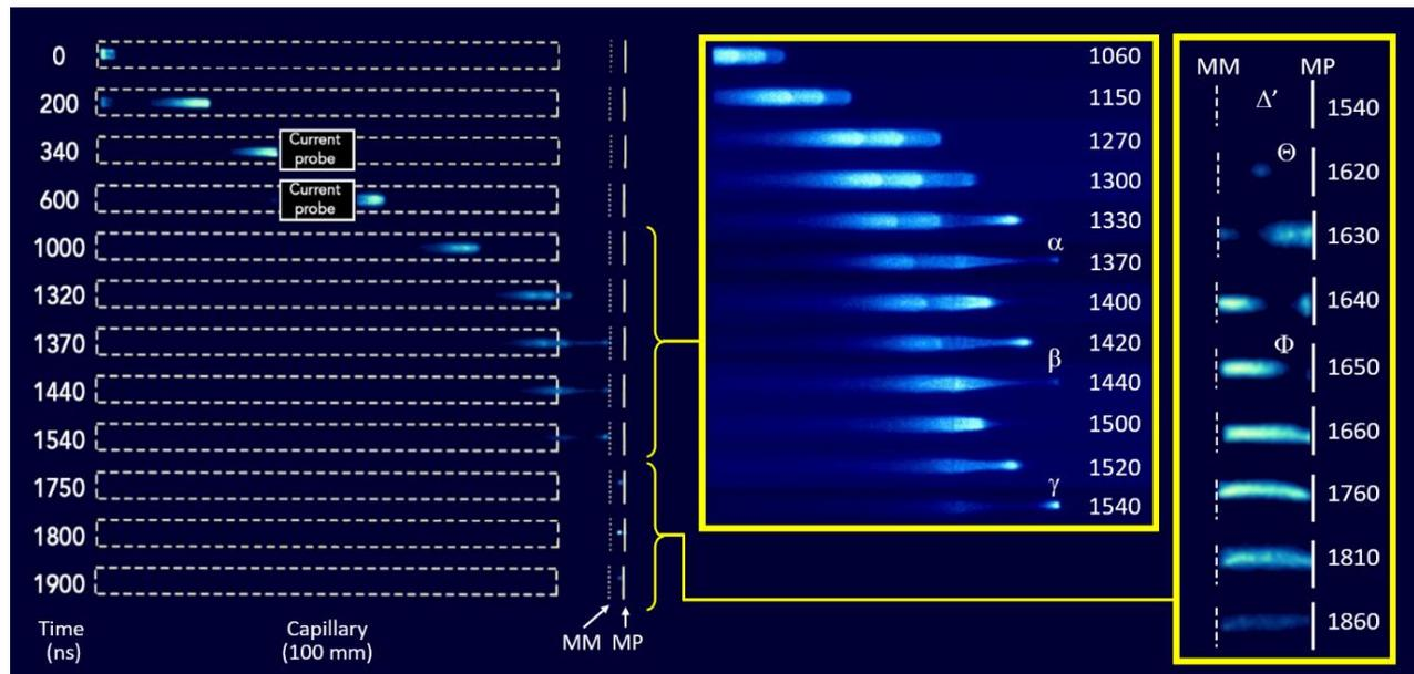
Figure 6. Fast ICCD pictures of positive guided streamers ( $\Omega = 3$ ) propagating in the CHEREL's capillary, then interacting with ambient air, metal mesh (MM) target at floating potential and metal plate (MP) target connected to  $R=1.5 \text{ k}\Omega$  that is grounded ( $A = 5 \text{ kV}$ ,  $f_{rep} = 5 \text{ kHz}$ ,  $D_{cycle} = 10\%$ ).
