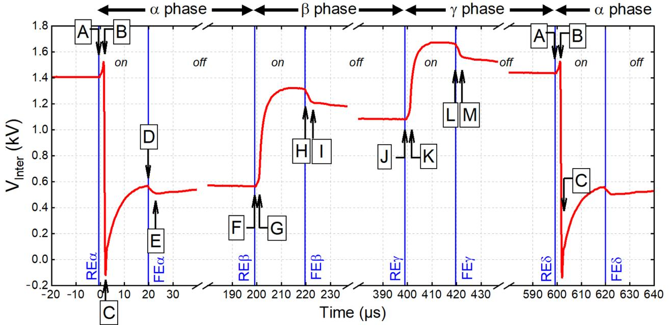
Figure 15. Time profile of the voltage measured in the inter-target region. The three phases correspond to the self-organization of three guided streamers ( $A = 5 \text{ kV}$ ,  $f_{\text{rep}} = 5 \text{ kHz}$ ,  $D_{\text{cycle}} = 10 \%$ ). RE and FE stand for rising edge and falling edge, respectively.
