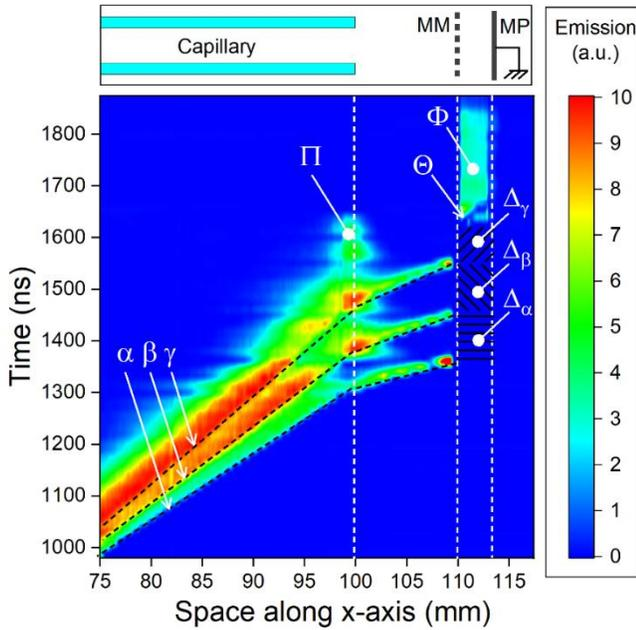
**Figure 7.** Space-time emission diagram obtained from fast ICCD imaging to highlight the self-organized guided streamers ( $\alpha$ ,  $\beta$ ,  $\gamma$ ) and decipher their mechanisms of propagation and interaction with MM and MP targets. II: residual surface discharge,  $\Delta$ : dark domains where leaders are assumed to be formed,  $\Theta$ : primary ionizing event in the inter-target region,  $\Phi$ : filamentary discharge.
