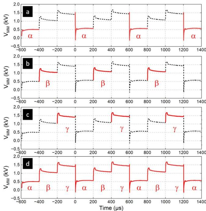
**Figure 8.** Time profiles of the voltage measured in the MM target considering (a)  $\alpha$ -phase highlighted, (b)  $\beta$ -phase highlighted, (c)  $\gamma$ -phase highlighted, (d) all phases highlighted. Schematic view of a train of (e)  $\alpha$ -streamers, (f)  $\beta$ -streamers, (g)  $\gamma$ -streamers. (h) Fast ICCD imaging picture of three self-organized guided streamers trains.
