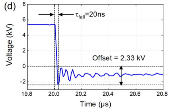
**Figure 2.** (a) Ideal positive square pulse, (b) real positive square pulse obtained with the HV power supply, (c) enlarged view of the pulse rising edge to evidence  $\tau_{rise}$ , overshoot and ringing, (d) enlarged view of the pulse falling edge to evidence  $\tau_{fall}$  and backswing.
