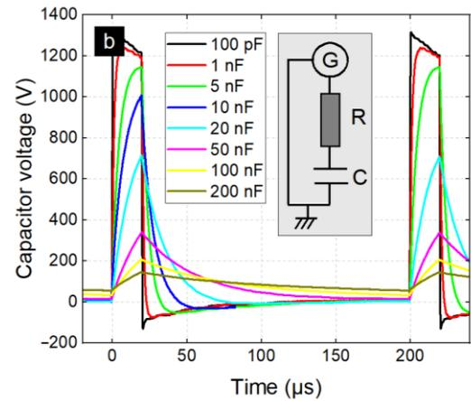
**Figure A1. (a) Capacitor voltage vs. rising time of a theoretical series RC circuit, (b) Time profile of capacitor voltage in a series RC circuit supplied with high-voltage nanopulse generator,  $A = 5000\text{ V}$ ,  $f = 5\text{ kHz}$  and  $D_{\text{Cycle}} = 10\%$ .**
