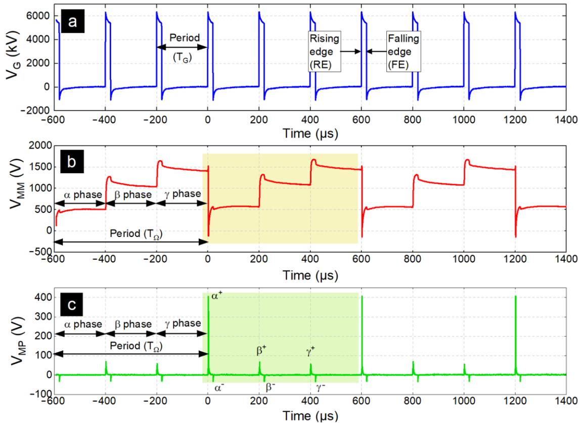
Figure 11. Time profiles of (a) the voltage delivered by the generator with the following set parameters:  $A = 5$  kV,  $f_{rep} = 5$  kHz,  $D_{cycle} = 10\%$ , (b) the voltage measured on the metal mesh target, (c) the voltage measured on metal plate target.
