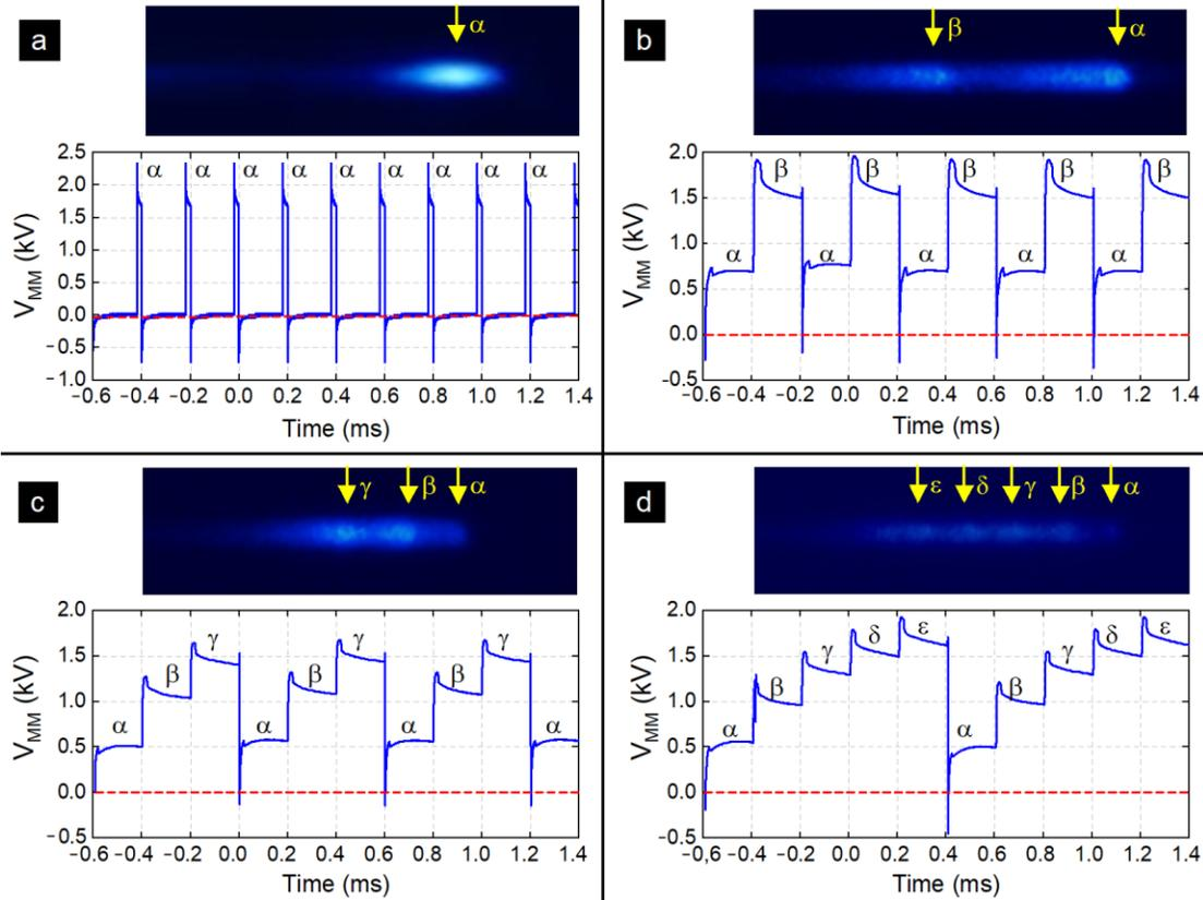
**Figure 5.** Spatial profiles of self-organized guided streamers measured by fast ICCD imaging and time profiles of the voltage measured on the MM target for (a)  $\Omega = 1$ , i.e., no self-organization, (b)  $\Omega = 2$ , (c)  $\Omega = 3$  and (d)  $\Omega = 5$ . The symbols  $\alpha$ ,  $\beta$ ,  $\gamma$ ,  $\delta$  and  $\epsilon$  represent the self-organizing states in order of appearance.
