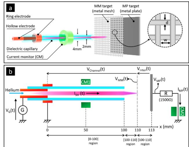
**Figure 1. (a)** CHEREL-MM-MP configuration. The CHEREL (Capillary with inner Hollow Electrode and outer Ring Electrode) generates a jet of cold plasma that interacts with MM (metal mesh target) and MP (metal plate target) placed in series, **(b)** Equivalent electrical schematics of **(a)** including voltage generator, electrical probes and resistor for electrical characterizations.
