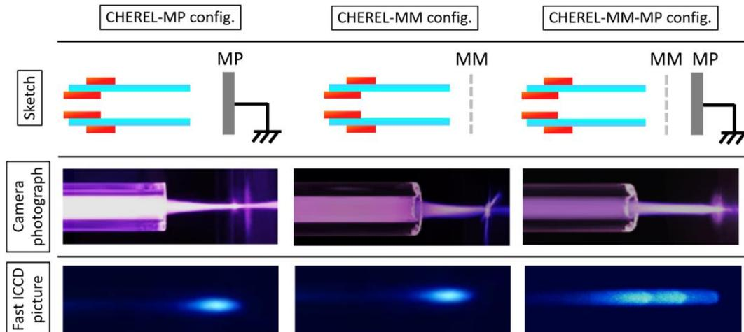
**Figure 3.** Pictures obtained by digital photography and by fast ICCD imaging, considering the CHEREL-MP configuration (train of repeated guided streamers), the CHEREL-MM configuration (train of repeated guided streamers) and the CHEREL-MM-MP configuration (train of self-organized guided streamers).
