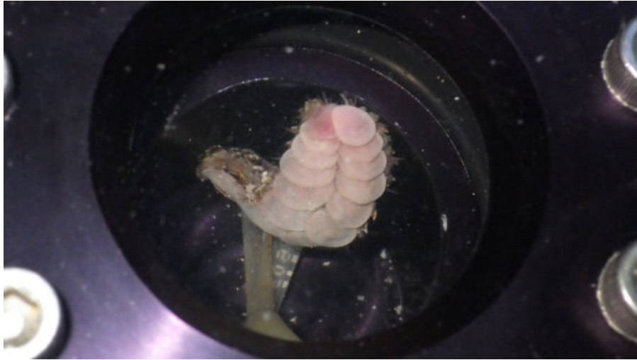
Figure 1: A specimen of the species Levensteiniella raisae in a small PAXDA pressurized aquarium under 150 bars of pressure.
