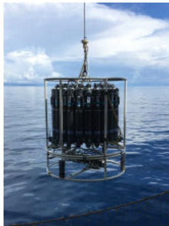
Figure 1. Deployment of the CTD-rosette fitted with 24 Niskin bottles, 2 Seapoint Turbidimeters, a pH and Eh sensor.
