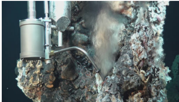
Figure 8: example of hot fluid sampling with a titanium syringe. © Ifremer – Chubarc 2019 Cruise.
