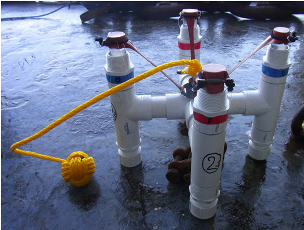
Figure 18: Tube-trap unit ready for deployment
