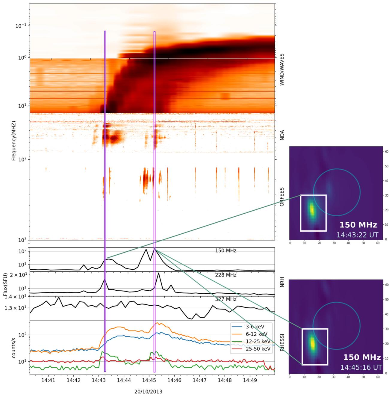
**Fig. 4.** Same as figure 3 for the event selected on 20 October 2013. The HXR data is from RHESSI. Two events are selected and considered in the study during the period plotted. The positions of the type III sources at 150 MHz for the two events are plotted on the right.
