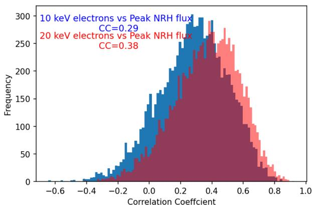
**Fig. 10.** Frequency distribution of correlation coefficient between the type III peak radio flux at 150 MHz and the number of electrons above 10 and 20 keV. The blue distribution corresponds to 10 keV electrons while the red distribution corresponds to 20 keV electrons. 10000 trials were conducted with 30 data points per sample.
