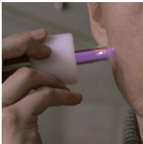
Figure 1. Application of a cold helium plasma jet on the skin. © GREMI, University of Orléans, CNRS
