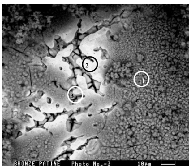
Fig. 1 – SEM image of the B66 bronze covered with a synthetic patina formed by galvanostatic method
