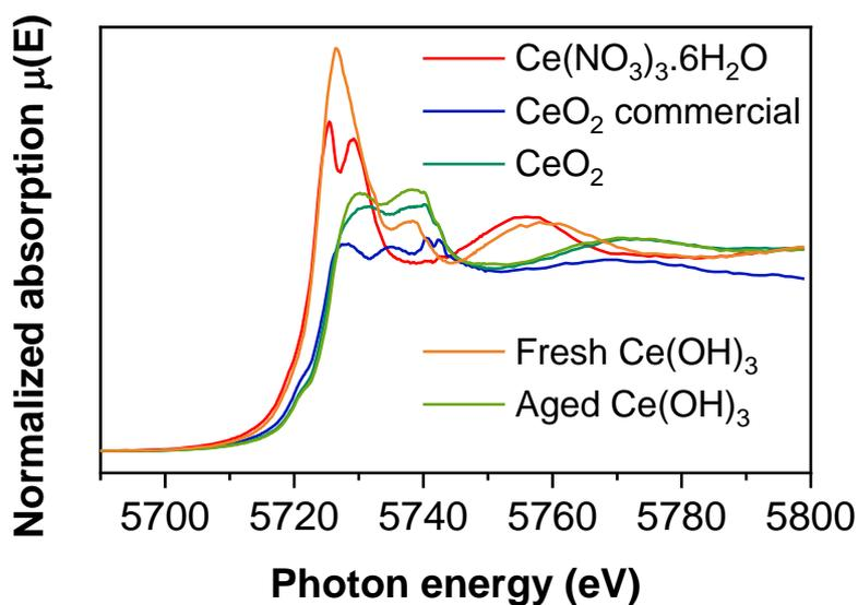
**Figure 3.** Ce L<sub>III</sub>-edge XAS spectra of commercial Ce(NO<sub>3</sub>)<sub>3</sub>·6H<sub>2</sub>O, commercial CeO<sub>2</sub>, CeO<sub>2</sub> nanorods, and of fresh and aged Ce(OH)<sub>3</sub>, measured as pellets in graphite.
