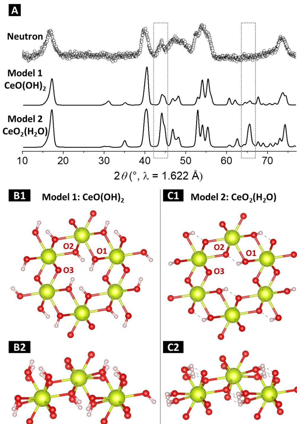
**Figure 5.** (A) Neutron Powder Diffraction (NPD) data of aged  $\text{Ce}(\text{OH})_3$  (up) and calculated patterns for models 1 (middle) and 2 (bottom). Acquisition at a wavelength of  $1.622 \text{ \AA}$ . Crystal structures of (B) model 1  $\text{CeO}(\text{OH})_2$  and (C) model 2  $\text{CeO}_2(\text{OH})$ , viewed along c-axis (B1, C1) or from a tilted angle (B2, C2) (Ce, O and H are represented as yellow, red and white balls, respectively, and dotted lines indicate H-bonding).
