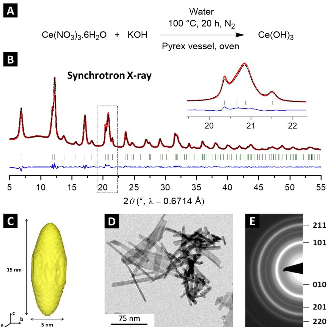
**Figure 1. Hydrothermal synthesis of  $\text{Ce}(\text{OH})_3$  nanoparticles.** (A) Reaction conditions. (B) Rietveld refinement XRD pattern (red: experimental data, black: calculated pattern, blue: difference, green bars: Bragg positions) with zoom on the  $[20-22]^\circ$  region. (C) Shape of the crystallites as deduced from the Rietveld refinement. (D) TEM image and (E) corresponding SAED pattern.
