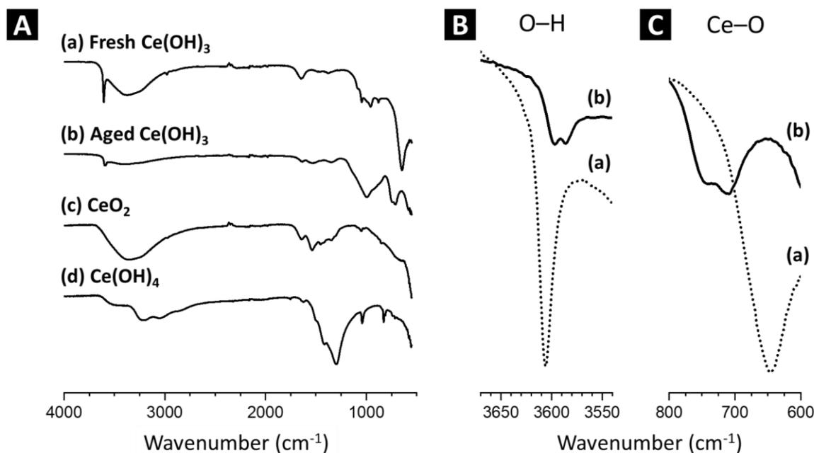
**Figure 6.** (A) ATR-FTIR spectra of (a) fresh  $\text{Ce(OH)}_3$ , (b) aged  $\text{Ce(OH)}_3$ , (c)  $\text{CeO}_2$  and (d) commercial  $\text{Ce(OH)}_4$ . Zooms on the (B) O–H and (C) Ce–O regions.
