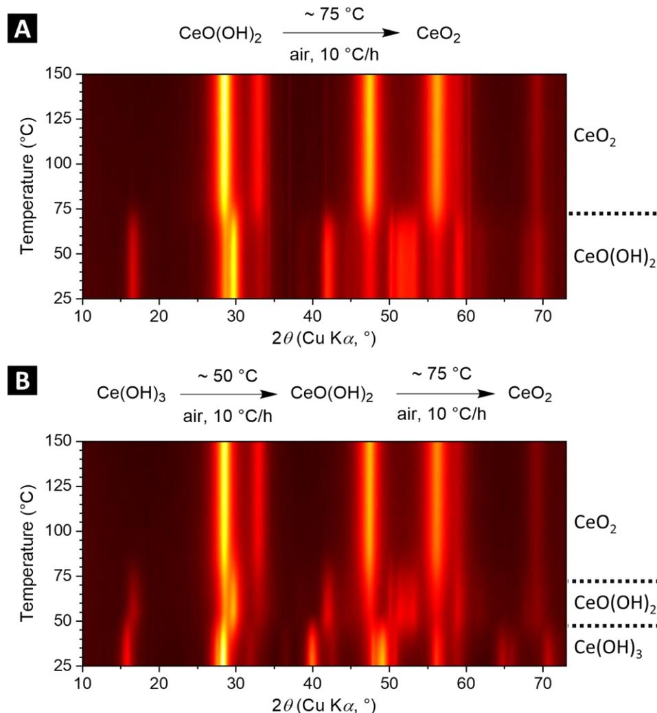
**Figure 7. *In situ* thermodiffraction experiments performed in air at a heating rate of 10 °C/h: calcination of (A) CeO(OH)<sub>2</sub> and (B) Ce(OH)<sub>3</sub>.**
