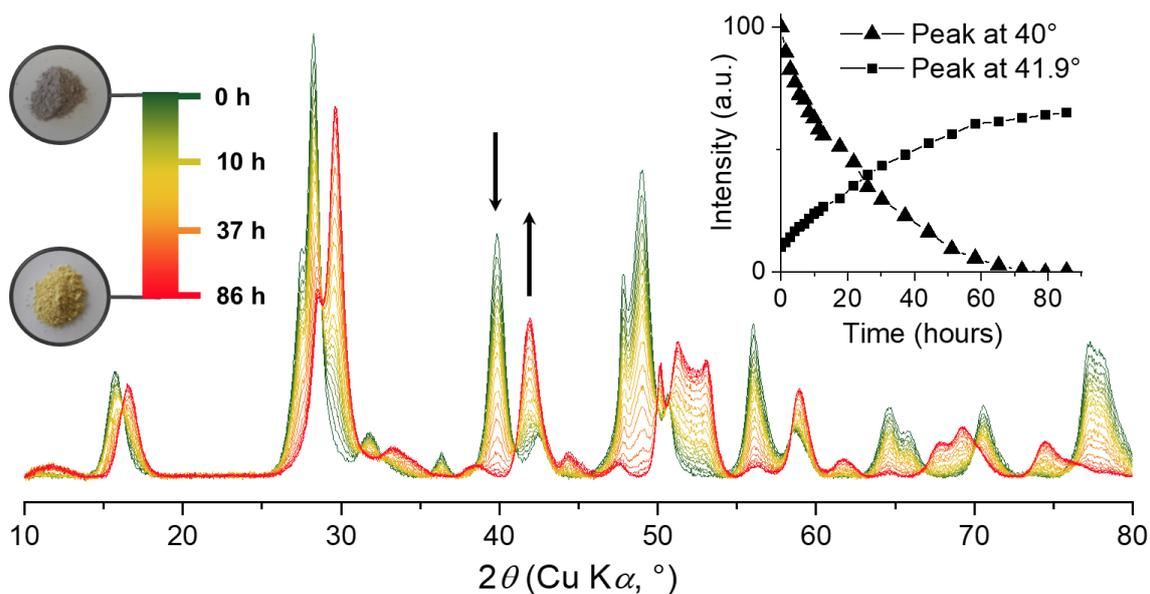
**Figure 2.** X-ray diffractograms of  $\text{Ce}(\text{OH})_3$  during aging in air. Inset: intensity of the (201) peak of  $\text{Ce}(\text{OH})_3$  (at  $40^\circ$ ) and aged  $\text{Ce}(\text{OH})_3$  (at  $41.9^\circ$ ) with time.
