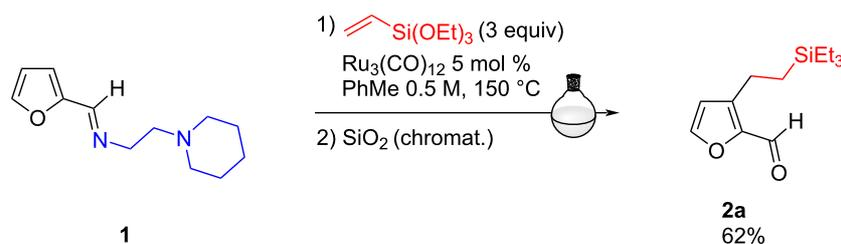
**Scheme 2:** C3-alkylation of bidentate imine **1** performed in batch.
