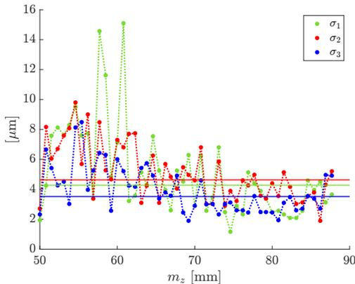
Fig. 9: Standard deviation  $\sigma_i$  of the time of flight measurement  $T_i$  along the 3D path, in water without the skull plate phantom. The horizontal lines give the median value of  $\sigma_i$  along the path.
