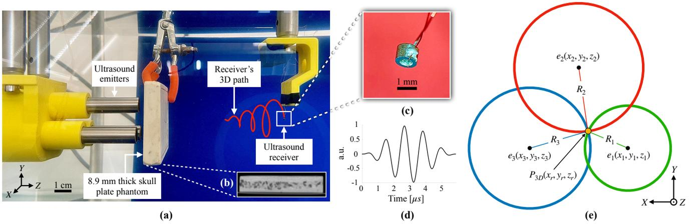
**Fig. 1:** (a) Picture of the experimental setup. (b) CT scan slice of the skull plate phantom (logarithmic inverse table). (c) Piezoelectric sensor used as ultrasound receiver. (d) Reference signal received on the sensor when excited by the emitters. (e) Illustration of the trilateration method in the XY plane. The colored radii correspond to the measured emitter-receiver distances.
