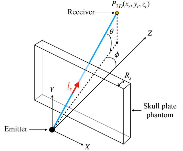
**Fig. 4:** Path of ultrasound from the emitter to the receiver, in water (in blue) and through the plate (in red). The receiver forms a lateral angle  $\phi$  and an elevation angle  $\theta$  relative to the emitter's coordinate frame. The vector  $\underline{l}_s$  approximates the effective path crossed by ultrasound in the plate before reaching the receiver.
