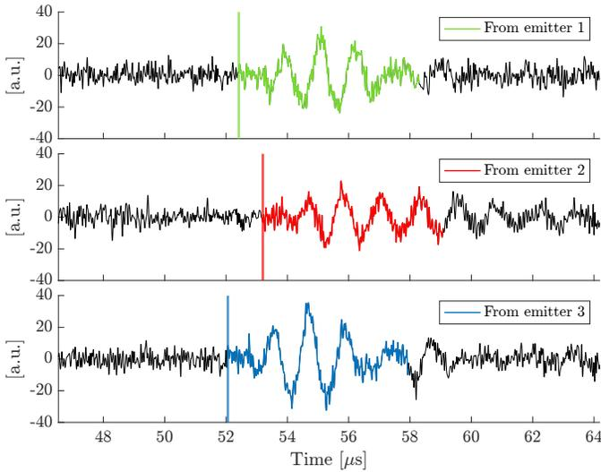
**Fig. 3:** Signal received from each emitter, through the skull plate phantom, at the motor's coordinate position [3.2 –7.3 80.0] mm. The time of flight  $T_i$ , measured by cross-correlation, is marked by a vertical line.
