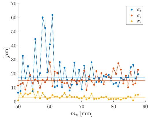
Fig. 10: Standard deviation  $\sigma_j$  of the  $j$ -coordinate measurement along the 3D path, in water without the skull plate phantom. The horizontal lines give the median value of  $\sigma_j$  along the path.
