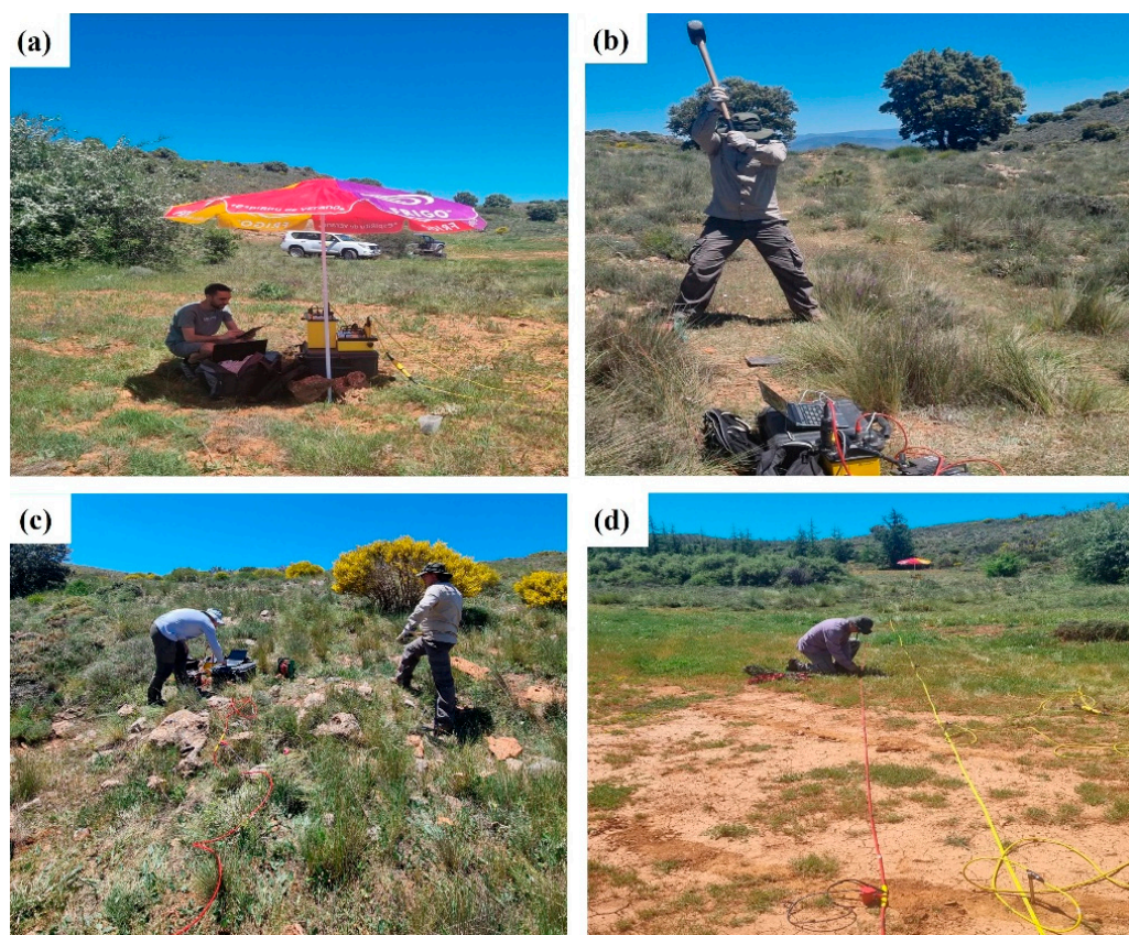
Figure 3. Visual documentation of equipment and operations in the field. (a) ERT survey using SuperSting R8 equipment from AGI. (b) Executed hammer blow (the shot) to generate seismic waves in an SRT survey. (c) SRT survey using SUMMIT II Compact equipment from DMT. (d) Checking of the electrodes (ERT surveys) and geophones (SRT surveys) for data acquisition.
