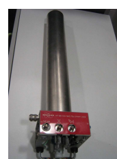
1 H-X CP-MAS Bruker ssNMR probehead suitable for 7mm rotors
