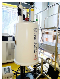
Ultraspeed 300WB Avance III Bruker ssNMR magnet
