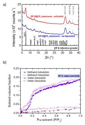
Figure 2. a) In-plane XRD patterns of ZIF-8@10\_exposures, as deposited (in blue) and after activation (in red), and a reference ZIF-8 signal from the data bank of DIFFRAC.EVA software (in black). b) Adsorption and desorption methanol and water isotherms obtained by ellipsometry porosimetry at room temperature (22°C) of the activated ZIF-8@10\_exposures.
