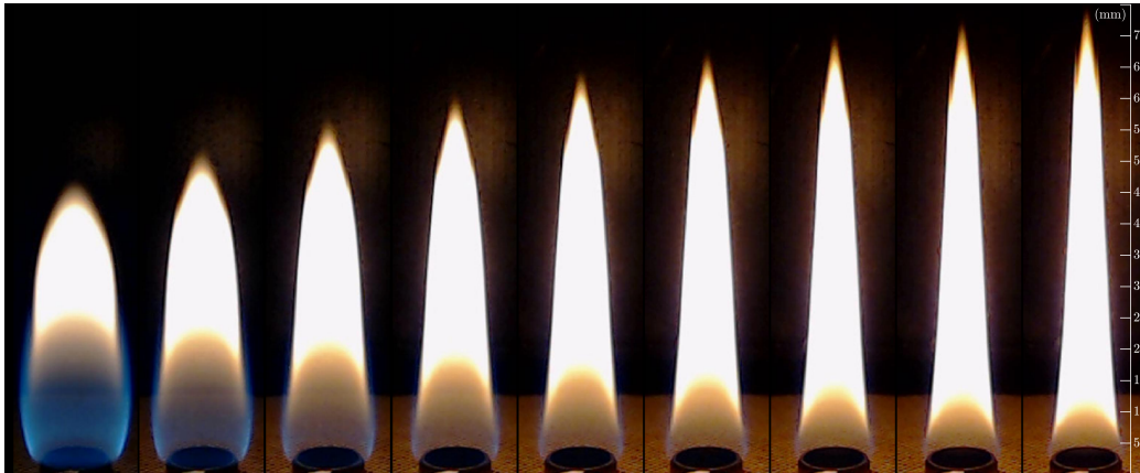
Figure 1: Pictures of the investigated flames. From left to right the pressure varies from 0.2 bar (flame E02) to 1 bar (flame E10).
