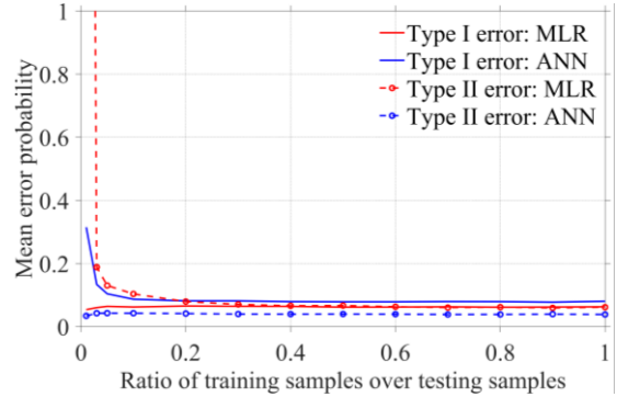
Fig. 10. Influence of the training data set size on type I and II error probabilities.
