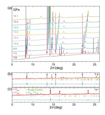
FIG. 1. a) X-ray diffraction patterns of GaGeTe as a function of pressure. While the  $R\overline{3}m$  structure remains unchanged till 15 GPa, at 16.1 GPa a new structural phase appears. b) LeBail fit to the data at 7.5 GPa with the  $R\overline{3}m$  structure. c) LeBail fit to the data at 16.1 GPa with the P3m1 structure. The sharp Bragg peaks (Grey solid circles) are from the crystallization of the pressure transmitter (Neon).
