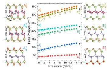
FIG. 3. The variation of the Raman modes with pressure. The measured frequencies (solid circles) are compared to the calculated *ab initio* values (empty circles). The side panels show the atomic movements of the corresponding zone center phonons. Three modes with out-of-plane vibrations of atoms ( $A_g$  symmetry) and three more with in-plane vibrations of atoms ( $E_q$  symmetry) can be observed.
