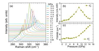
FIG. 6. a) Variation of the  $E_g^3$  mode with pressure. The  $E_g^3$  mode for the Ge plane ('germanene') is analogous to the graphene G mode. b) Intensity and c) Linewidth variation of the  $E_q^3$  mode.
