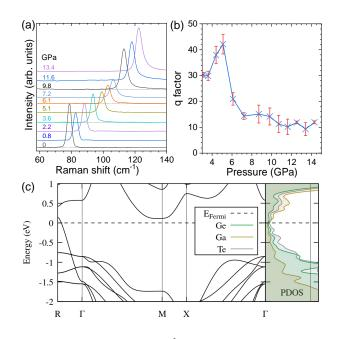
FIG. 5. a) Variation of the  $A_g^1$  mode with pressure showing the mode becoming wider and asymmetric at higher pressure. The baseline is shown for a few pressures b) q factor (signalling asymmetry) extracted from a Breit-Wigner-Fano line shape fit. c) Electronic structure and partial density of states at 6 GPa
