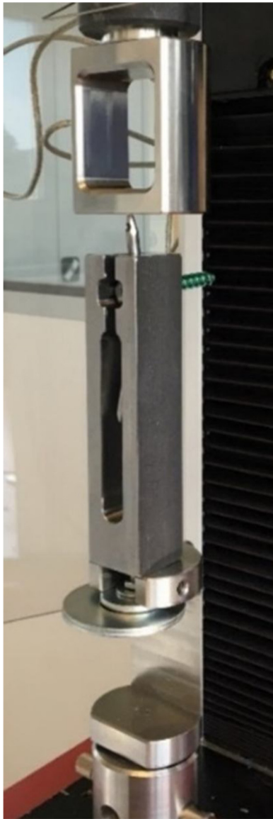
Fig. 4. Axial gripping capacity test set-up.
