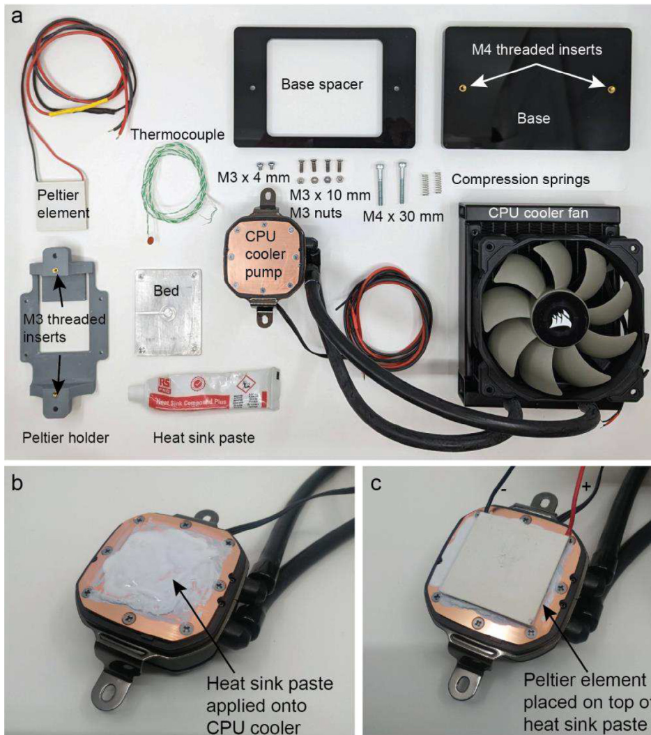
Fig. 2. Required parts for the bed build (a). Application of thermal compound to top of cooler block (b). Peltier element placed on top of thermal compound with cold side facing up (location of red and black wires used as reference) (c). (For interpretation of the references to color in this figure legend, the reader is referred to the web version of this article.)
