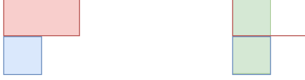
Fig. 5: The join between the red and blue rectangles on the left is not exact, however it is possible to under-approximate the red rectangle along the x-axis with the intersection between the x components of the two rectangles (case (6a)). The result can be joined exactly yielding the rectangle in green on the right.
