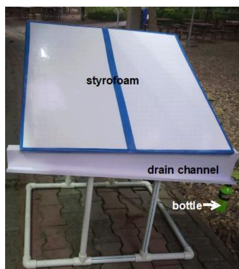
Figure 2. The DIY dew condenser unit (with transparent polyethylene sheet).
