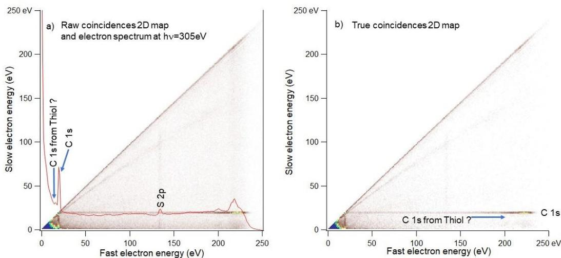
Fig. 3: Coincident electron spectrum at  $h\nu=340$  eV about 50 eV above the C(1s) ionisation thresholds with 30V retardation. a) raw coincidence 2D map and electron spectrum. b) true coincidence 2D map after subtraction of random coincidences deduced from the electron spectrum.
