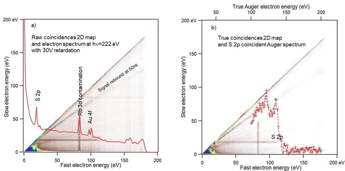
Fig. 2: Coincident electron spectrum at  $h\nu = 222$  eV about 50 eV above the S(2p) ionisation thresholds with 30 V retardation. a) raw coincidence 2D map and electron spectrum. b) true coincidence 2D map after subtraction of random coincidences deduced from the electron spectrum. The S2p coincident Auger spectra is shown with the good energy scale.
