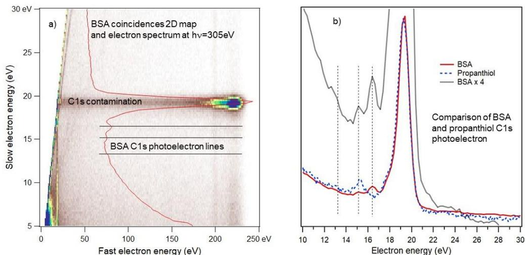
Fig. 4: a) Coincident electron spectrum at  $h\nu=340$  eV about 50 eV above the C(1s) ionisation thresholds with 30 V retardation for BSA (Bovine Serum Albumin). b) comparison of the C1s photoelectron spectra for BSA and 1-propanethiol .
