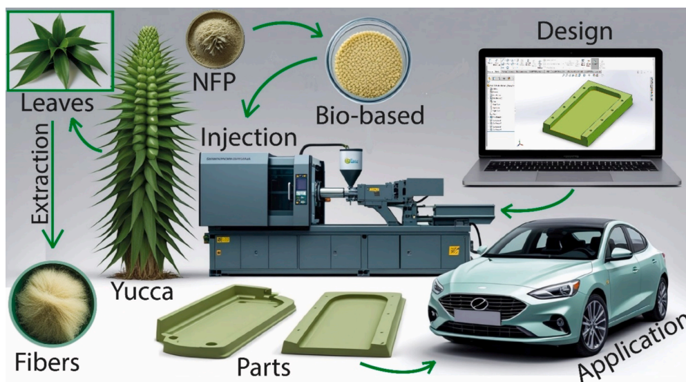
Fig. 1. - Overview of the manufacturing stages of injection-molded bio-composites for automotive components. (NFP is Natural Fibers Powder).
