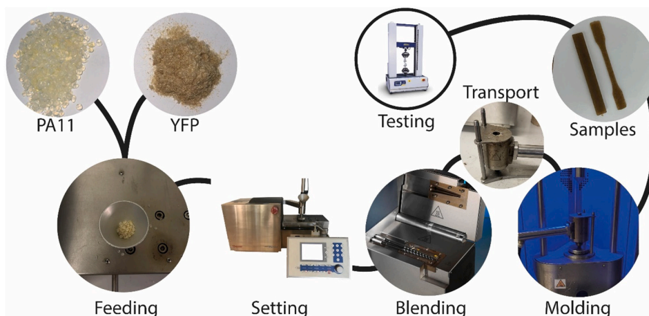
Fig. 2. Fabrication route of injection-molded PA11/Yucca composite specimens.
