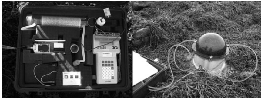
FIG. 2. Container with circuit of CO 2 analysis and data logger and benthic chamber with dark dome connected to the circuit on the Ascophyllum nodosum zone.
