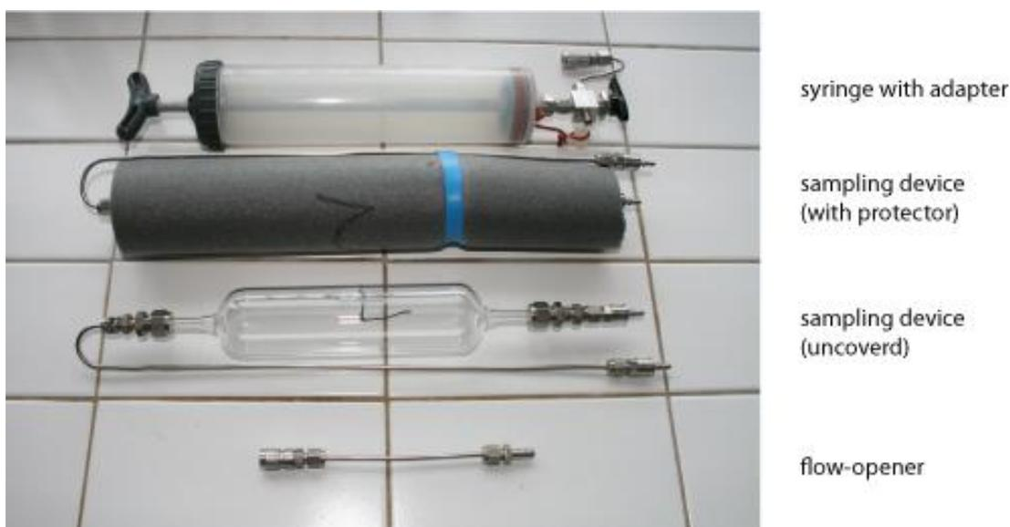
Figure 12. Sampling device (air), glass bulb and syringe.
