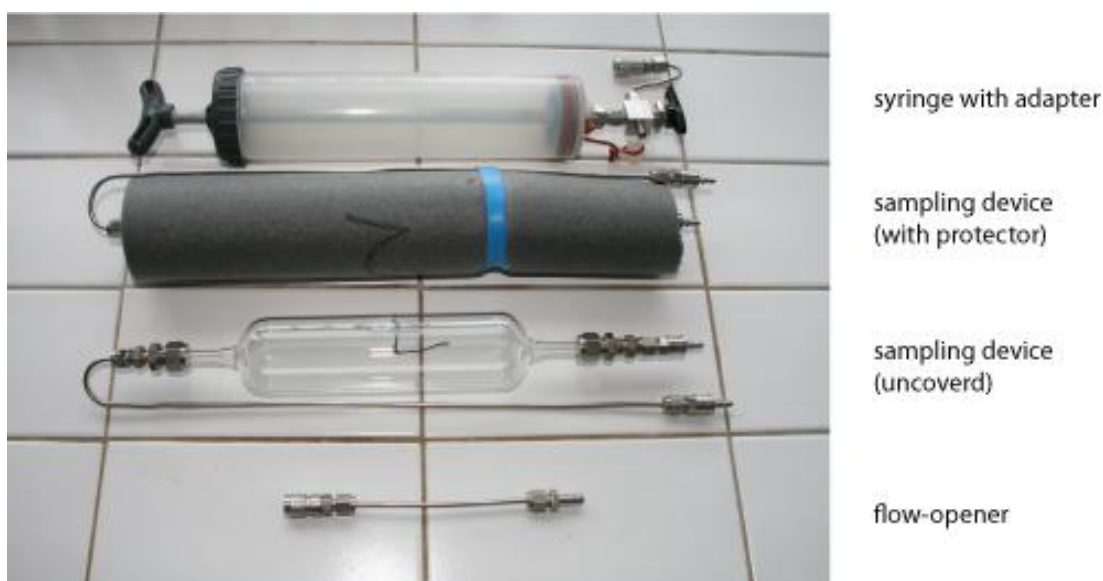
Figure 12. Sampling device (air), glass bulb and syringe.
