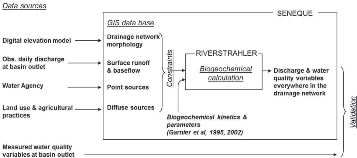
**Figure 5-2.** Representation of the Seneque/Riverstrahler model.
