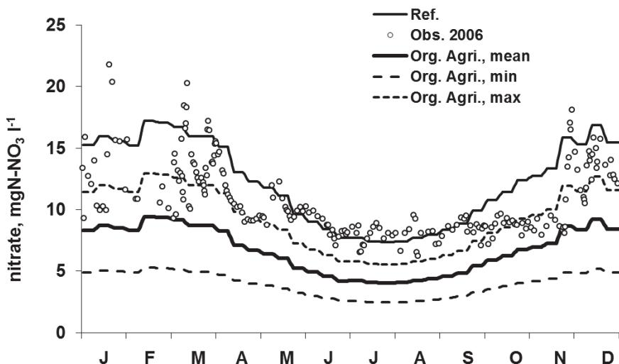
**Figure 5-8.** Seasonal variations of nitrate concentrations at the outlet of the Orgeval Basin, the year 2006 taken as example. A rather good agreement is obtained between the observations and the simulation for 2006. Compared to the reference simulation, the organic agricultural scenario shows a 45% decrease in annual mean nitrate concentrations (Org. Agri., mean). The amplitude of the response is shown with the exploration of the SD range (Org. Agri., min and max).
