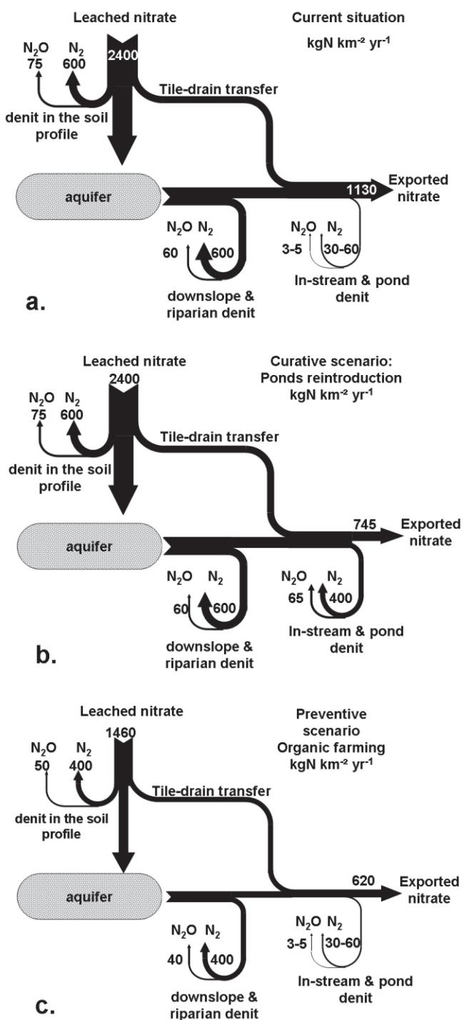
**Figure 5-5.** Summarizing budget of nitrate transfer and transformation and associated nitrous oxide emissions in the Orgeval Basin. Calculations are based on the average hydrology from 2006 to 2012. a) current situation based on measurements; b) scenario of pond reintroduction; c) scenario of organic farming.
