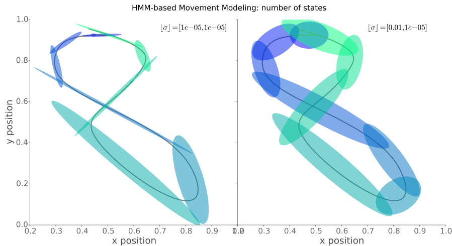
Figure 4.13: Influence of the regularization in HMM-based movement modeling. A model is trained using a single 2D movement example (solid gray line). The hidden states are represented by their 95% Confidence Interval Ellipse (from blue to green in the left-right order of the hidden chain). The figure represents the models learned with different values of the relative part of the regularization. Increasing the prior globally increases the variance over all states, ensuring a better generalization of the movement.
